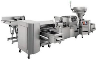
The automation solution comprises a VF 600/VF 800 vacuum filler, a PVLS 143 AL cutting line, a collating system and a collating belt
